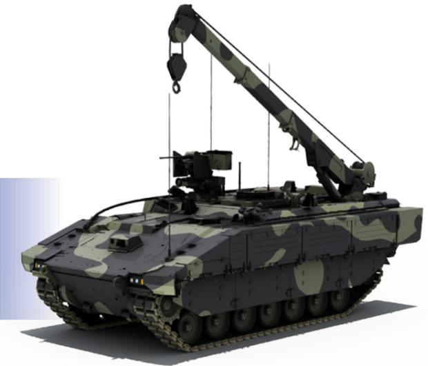
The **APOLLO** variant will be used to tow battlefield damaged vehicles and lift heavy sub-assemblies.
